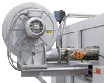
Cooling fan for accelerated cooling
