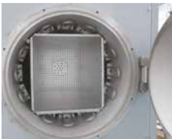
Inside heating in retort furnaces NRA ../06
