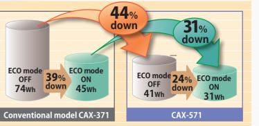
Measurement conditions: Set to 4°C at an ambient temperature of 25°C while centrifugation is stopped. (Rotors in use: CAX-571: TS-7C+7215-06) The values shown above are average values obtained by measuring the units.
