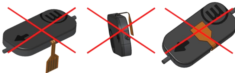
Figure 19 Important notes about the proper use of the flexible connector
