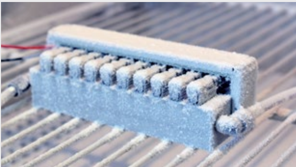
Laboratory simulation tests at lower temperatures to guarantee performances between 0 and 50°C
