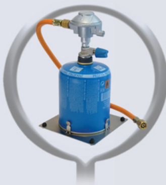
Safety adapter CV with integrated pressure regulator, gas leak protection, DVGW-tubing (0.5 m) and stainless steel stand for gas cartridges CV 470 / 270: Art.-No. 6.000.850 CV 300: Art.-No. 6.000.831
