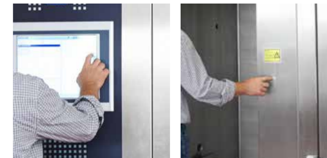
On walk-in chambers, additional safety buttons prevent people from being trapped.
