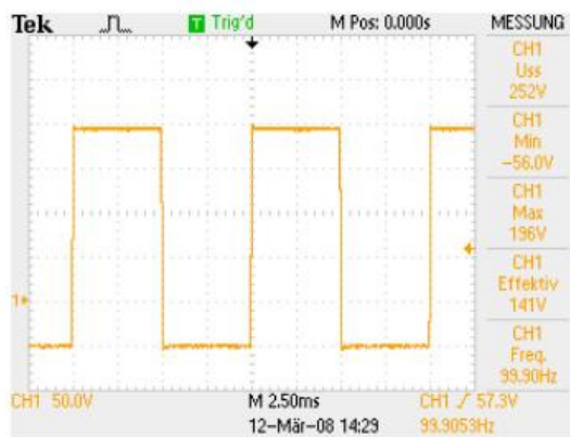
mpx, Rectangel-Signal, 250Vpp, 100Hz
