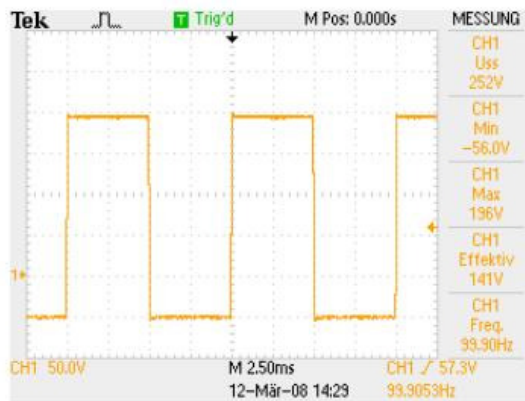
mpx, Rectangel-Signal, 250Vpp, 100Hz
