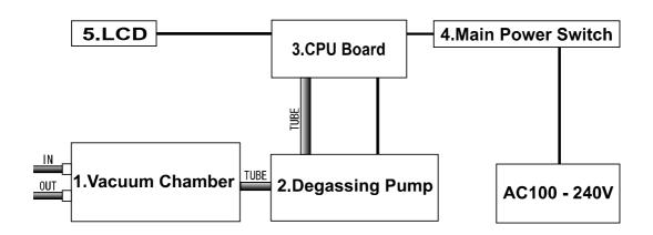
Vacuum Chamber The vacuum chamber contains densely packed membrane filters and maintains precise vacuum level with the degassing pump.
