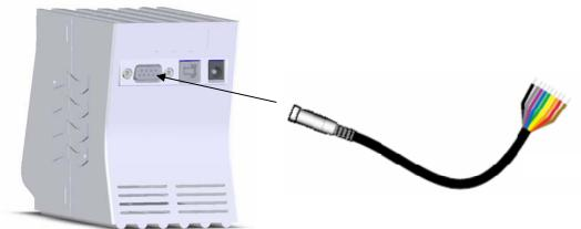
• Connect the interface cable wires to the controlling instrument contact closure as instructed below. The controlling instrument must have one contact closure output (event relay) for two-position valves and four contact closure outputs for multi-position valves.
