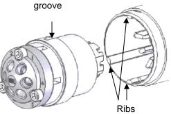
• Replace the spanner and tighten clockwise, (Hand tighten only, do not use wrenches on the spanner nut.)
