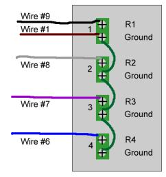
Fig 2. Wire connections for multi-position MX Series II Modules. Wire colors may vary.
