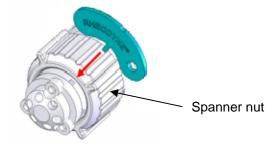
• Turn the Spanner nut counter clockwise until the Rapid Replacement Pod detaches from the MX Series II Module. (Do not use wrenches on the Spanner nut.)
