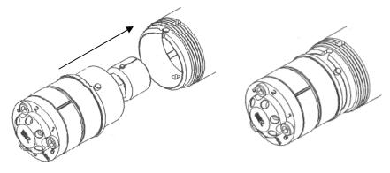
• Continue to rotate until the clocking pin aligns with the notch in the housing.
