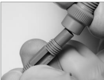
FIGURE 6 Set the capsule union on the inlet end of the column holder. Cover with an end cap and very loosely tighten.
