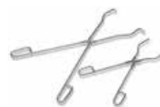
Various tongs for easy loading and unloading of the furnace.
