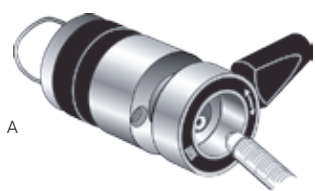
Figure 2 (A) Syringe fitted with Needle Port Cleaner (Part # 7125-054) loading a front-loading valve (model 7725); (B) loading a Loop Filler Port (Part # 7012)
