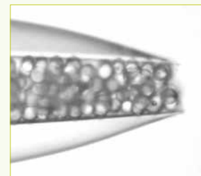
A magnified view of the fritted tip of the PicoFrit column (15 µm tip)
