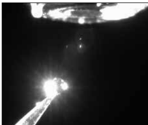
Droplet formation Spray voltage too low
