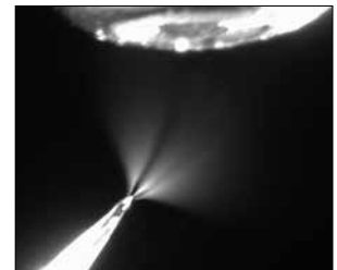
Split-Spray Spray voltage too high
