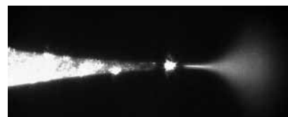
GlassTip with a 1.2 mm OD, 0.69 mm ID, and 2 μm tip spraying at 60 nL/min.
