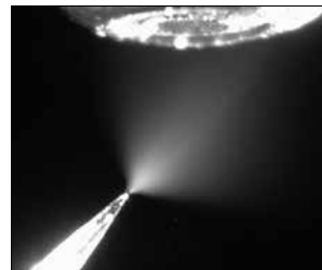
Perfect Plume Spray voltage is optimal
