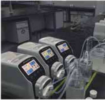
Laboratory chemical dosing
