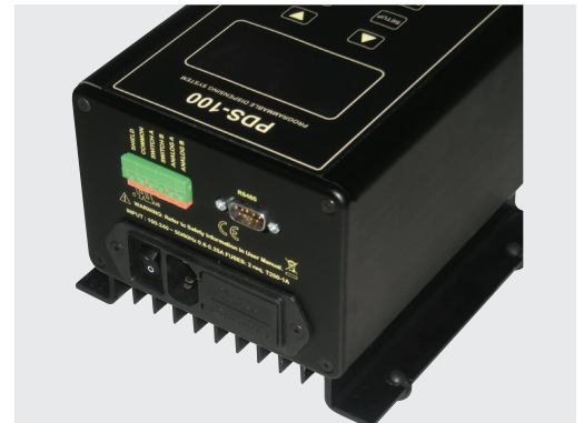
Selectable RS485, 4-20 mA, 0-5 V DC, and 0-10 V DC input for automatic control
