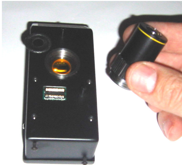
Objective and seat for fluorescence filter
