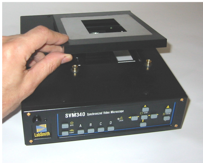
Removing the microscope stage
