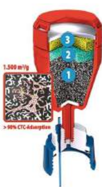
Fig. 2: The Safety Waste Caps contain three different types of activated carbon for additional safety: 1st layer adsorbs solvent vapours, 2nd layer binds alkalis, 3rd layer binds acids.
