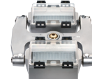
TS-41N Deep-well Platex4 4,500rpm : 3,150G Bucket, Adapter and Bucket Cover are Includud.
