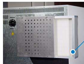
HEPA-filter, 0.3µm, Class H, Efficiency 99.95%
