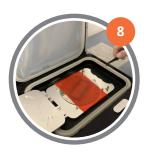
Ensure a thin PTFE sheet (red) is placed on top of the sandwich to avoid sticking to inside of the metal cover.
