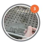
Remove one protective PTFE sheet from the Flexdym™ and place the Flexdym™ on the counter mold using tweezers.
