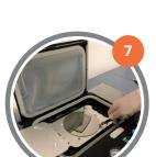
Using protective gloves & tweezers, place Mold-Flexdym-Counter mold sandwich in Sublym™ molding chamber.
