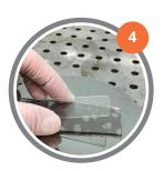
Remove the second protective PTFE sheet from other side of Flexdym™. Place the mold face down on the Flexdym™ sheet.
