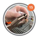
**Optional:** Use metal hole punch pliers to create inlet/outlet holes in the design.
