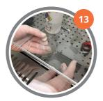
Gently remove the molded Flexdym<sup>™</sup> from the mold.
