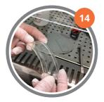
Cover both sides of the Flexdym™ with the protective PTFE sheets. Cut neatly around the molded design.
