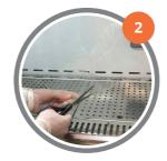
In a ductless fume hood, cut the Flexdym™ sheet using scissors, according to the size of your mold.
